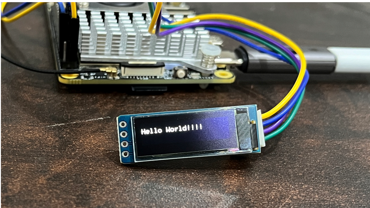
Fig. 5.22: Hello World!!!! on 128x32 OLED
