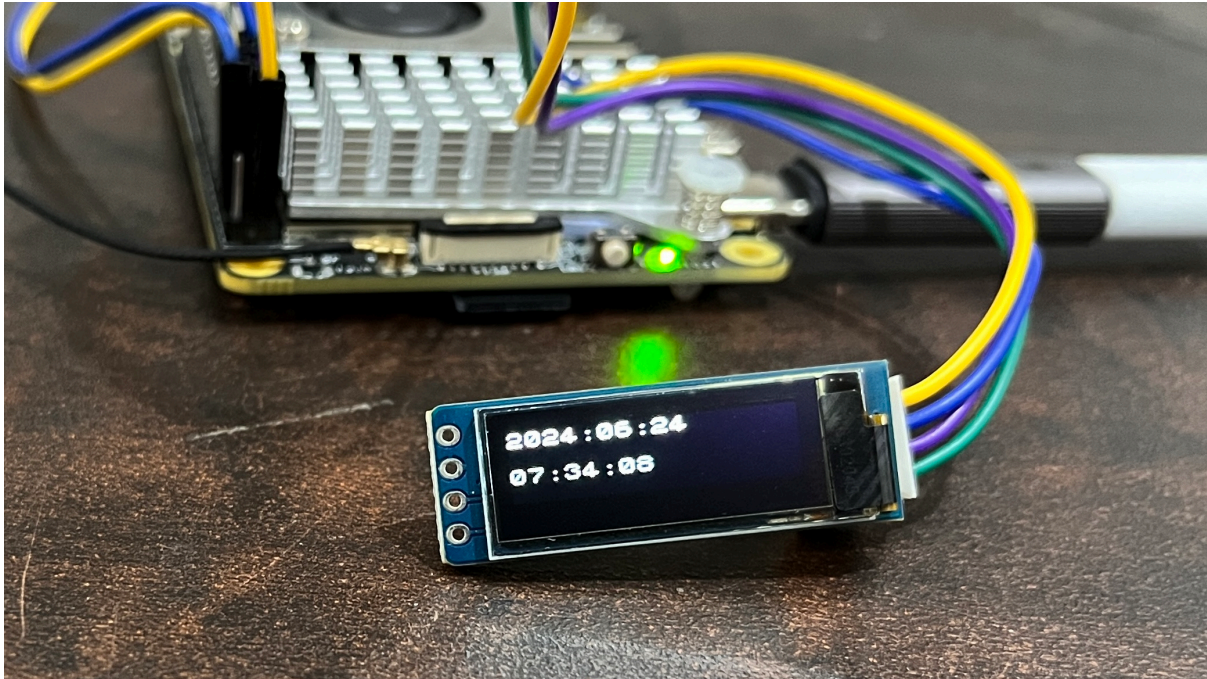
Fig. 5.24: Date &amp; Time on 128x32 OLED
